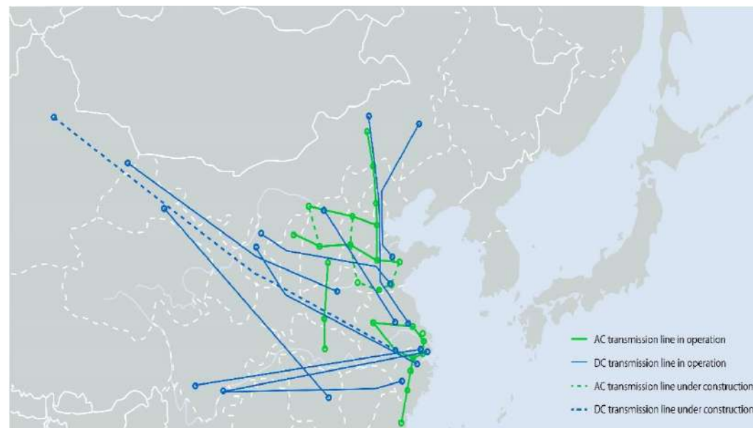
Figure 1: China SGCC's domestic ultra-high voltage transmission project
